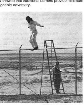
BILL INGRAM (2454) demonstrates stepladder launch over fence. No-touch technique means that fence sensors would not be activated by this type of intrusion.
